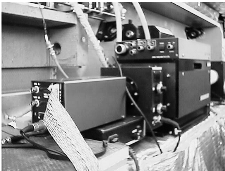
Figure 1: Streak Camera with \mu CP and CCD assembly.
